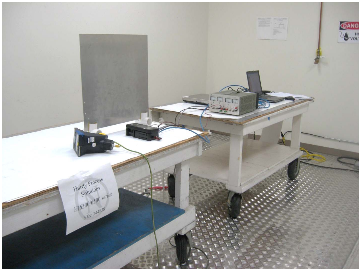
Photograph 6. ESD Test Configuration
