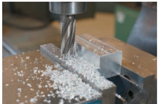
Figure J-52 Roughing end mill used to remove a large volume of material.
