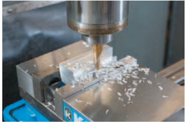
Figure J-50 Using an end mill to mill steps.
