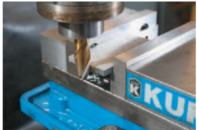
Figure J-51 Using an end mill to square stock.
