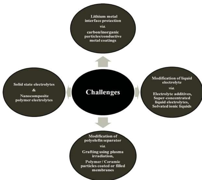
Fig. 6. Various strategies to suppress Li dendrite growth for improving the safety and cyclic stability of rechargeable lithium-metal batteries.
