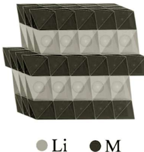
Fig. 6. Crystal structure of layered \text{LiMO}_2 cathode material (Reprinted with permission from [39]. Copyright (2015) American Chemical Society.
