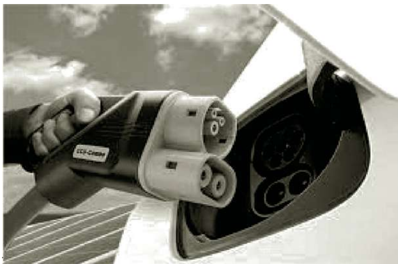
Fig. 5. SAE J3068 AC Depot Conductive charging.
