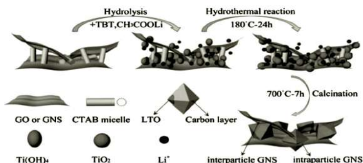
Fig. 1. Schematic illustration of the synthesis and structure of carbon coated LTO/graphene (C-LTO/G) architecture [51]. (Copyright © 2014 Elsevier)
