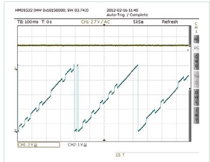
Figure 12. Pure phase modulation: amplitude shown in yellow, phase in blue.
