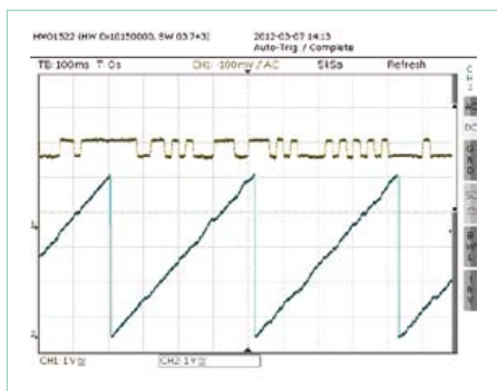
Figure 1. AM modulation: amplitude in yellow, phase in blue.
