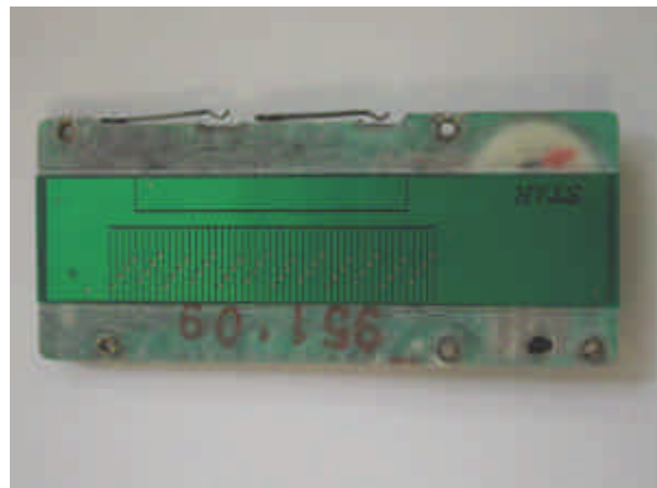
Fig. 4 the actual capacitive measuring sensors on the backside
