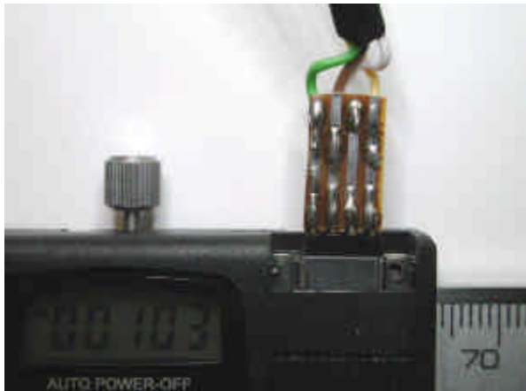
Fig. 12 calliper with plugged-in cable
