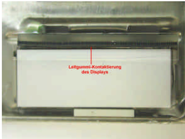
Fig. 5 Display with rubber connector
